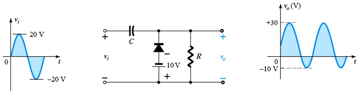
Figure 2.28: Clamping network with a sinusoidal input.
