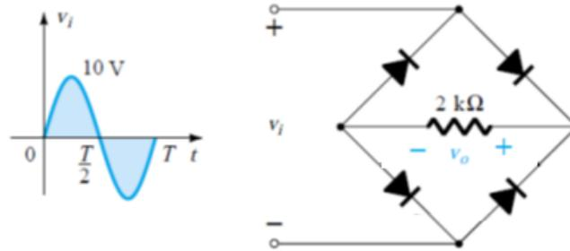
$v_i$  can be written as  $v_i = 10 \sin(\omega t)$ , 10 means the maximum input voltage.
