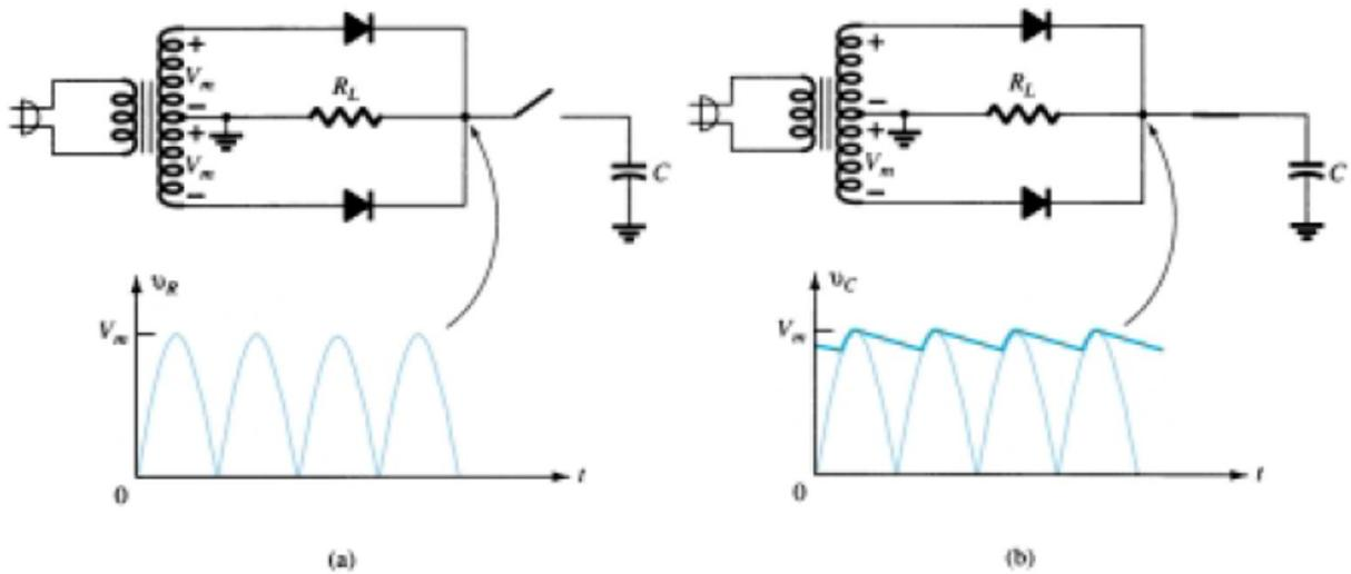
Figure 2.29: Full Wave rectifier with and without capacitor filter.
