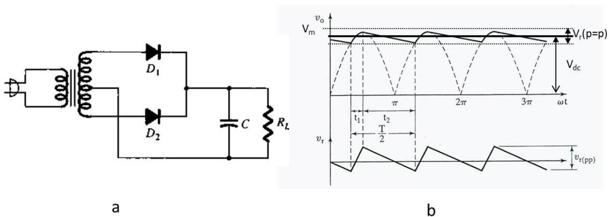
Figure 2.30: Capacitor filter: (a) capacitor filter circuit; (b) output voltage waveform..
