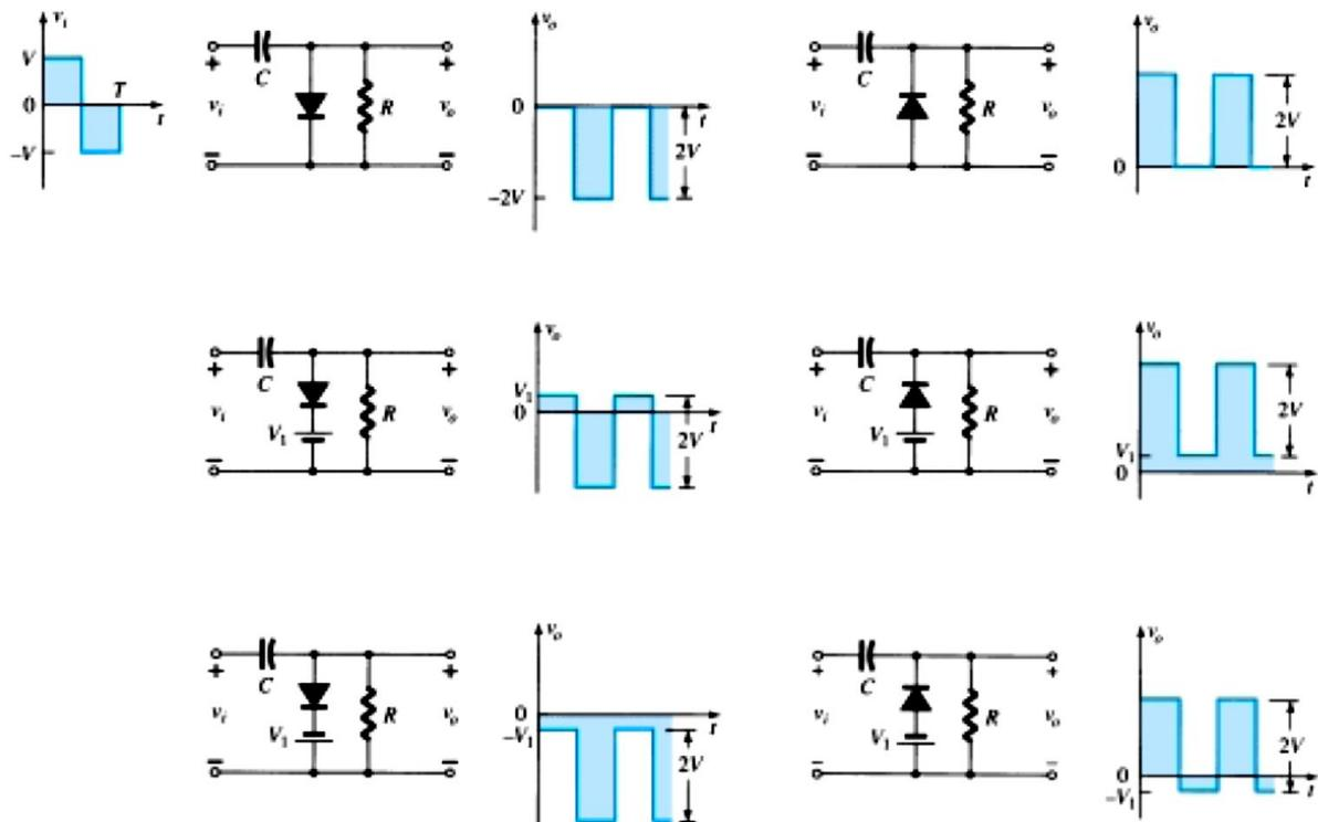
Figure 2.27: Clamping circuits with ideal diodes ( $5\tau = 5RC \gg T/2$ ).
