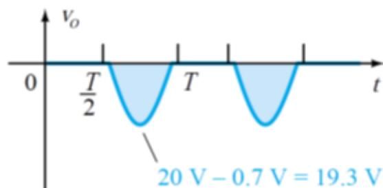
Figure 2.8: Effect of  $V_T$  on output.
