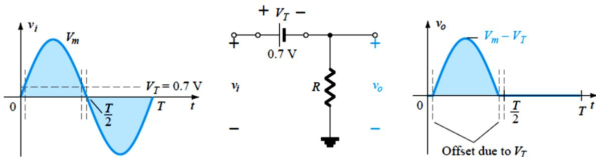
Figure 2.5: Effect of  $V_T$  on half-wave rectified signal.
