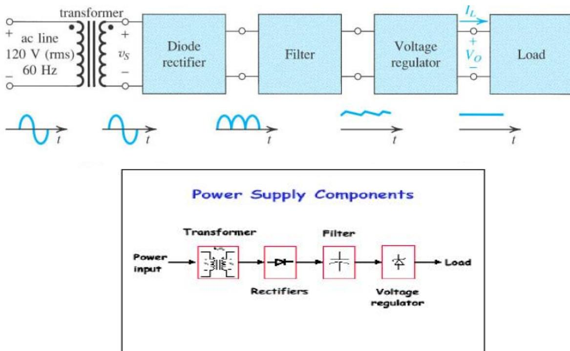
Figure 2.28: Typical Power supply configuration.
