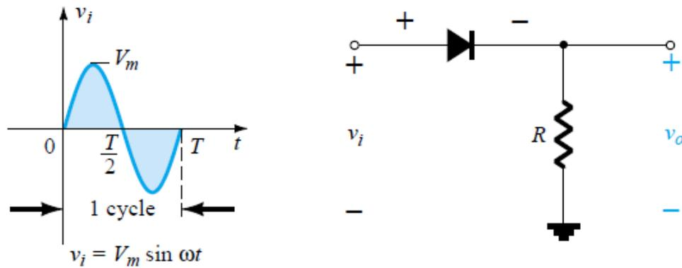
Figure 2.1: Half-wave rectifier.
