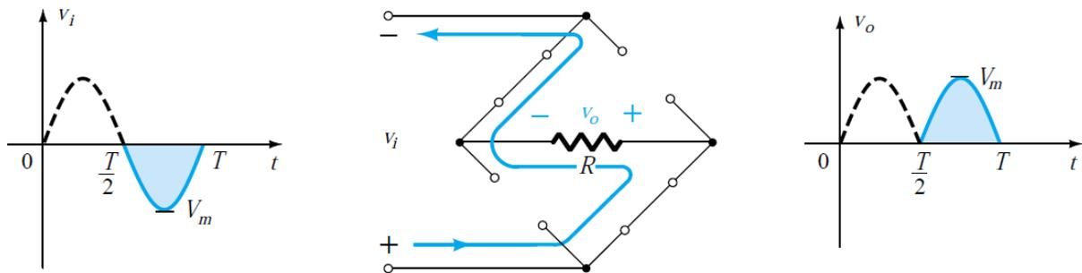
Figure 2.13: Conduction path for the negative region of  $v_i$ .
