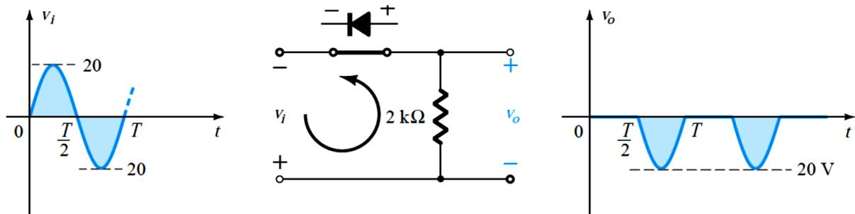
Figure 2.7: Resulting  $v_o$  for the circuit of the example.
