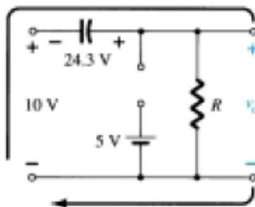
To compute  $v_o$ , apply KVL on the indicated loop:
