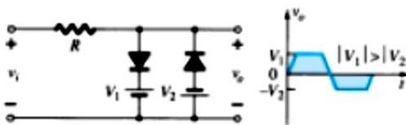
Figure : Clipping circuits.
